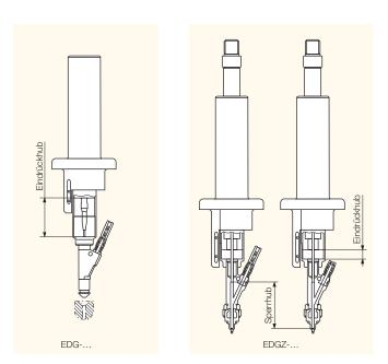
DEPRAG press-insertion devices for handheld applications excel through the ergonomic form of the handle and the high efficiency when connected to a suitable feeder.
