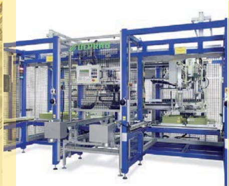
Screw assembly of a radiator grille
