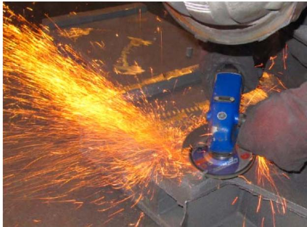
*Grinder equipped with a cup wheel*
