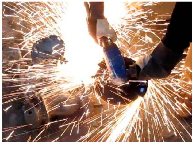
*DEPRAG Turbine Grinder used in a Foundry*
