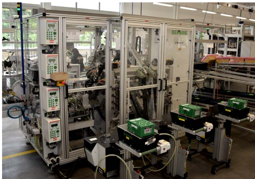
Station No. 1 – shown with the different feeders & hoppers
