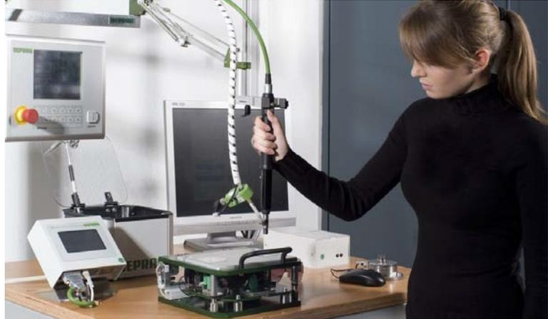
The new AST5 controller records the cycle results from the previous seven production days, and stores them for retrieval via the Ethernet connection. Additional advantages are the detailed graphical-display of the screwdriving curves, the integrated PLC-functions, as well as comprehensive analysis options. This ensures the successful traceability of the production steps, along with an optimal quality-management process.
