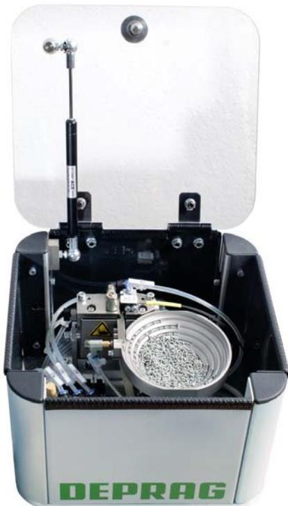
Furthermore, the AST5 provides the option to be combined with an automatic screwfeeding device. It is one thing to assemble such small screws within a reliable process, but quite another to automatically separate and feed them repeatedly to the screwdriver in a precise rhythm. DEPRAG introduces another innovation: The DEPRAG screwfeeder for micro-assembly operations, with a fill-capacity of just 0.05 liters!
