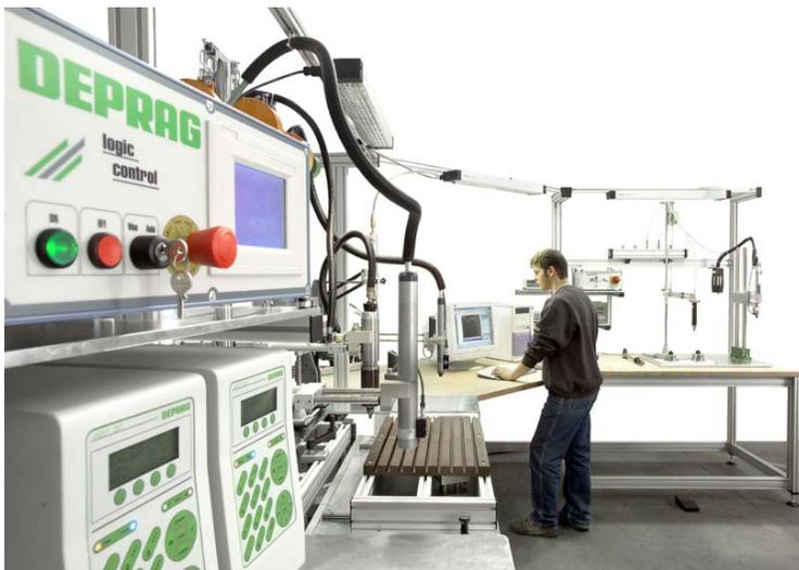
single part, meeting the highest requirements. The purpose of the screw in this process is to clamp the components tightly together so that they cannot be shifted by external forces. The achieved force is called pre-tension. The screw assembly has to remain within the range of defined tolerance limits: On the one hand, the achieved pre-tension must be sufficient to keep the component together, while on the other hand the screw and component should not be damaged by over tightening.
