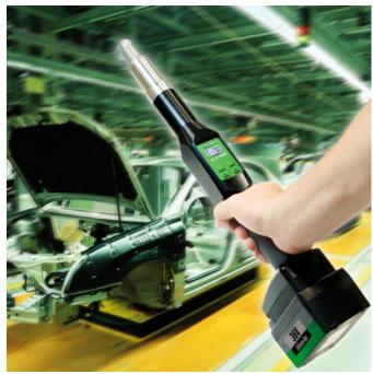
driven screwdrivers were not very convincing, mainly because of their short life span. However, the performance of today's battery-operated screwdrivers can no longer be compared with this old technology." The DEPRAG engineers decided in favor of the latest generation of Lithium-ion rechargeable batteries for this new screwdriver series.
