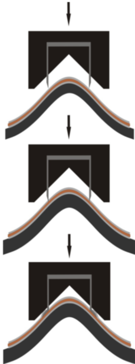
Direct Contact Spring Clip assembly via "Contact Mound"
