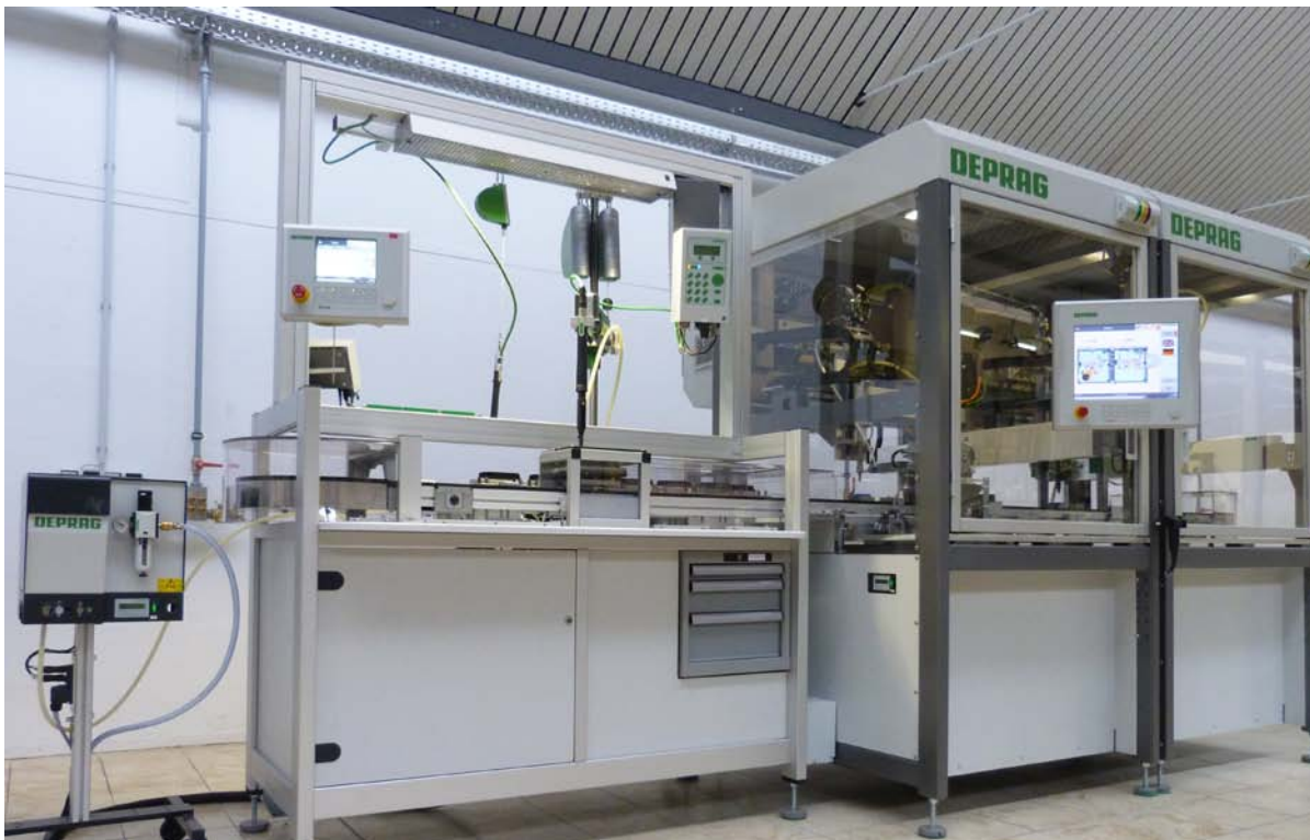
Full Workstation with Screwdriving, Screwfeeding and Part Fixturing
