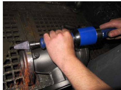
Application Example: Grinding a casted product a high speed with the DEPRAG-Industrial Turbine Inline Grinder GDST 100-280BX
