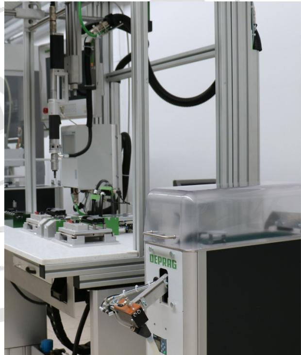
Sword feeders are used for the feeding of varied fasteners. Jürgen Hierold: "For this sector, we use feeding technology which fulfils the requirements of technical cleanliness. In contrast to vibratory spiral feeders, only low friction is generated during the transport of fasteners. In addition, at the points where friction can occur, vacuum fittings are connected. Damaging dirt particles are largely eliminated through suction."
