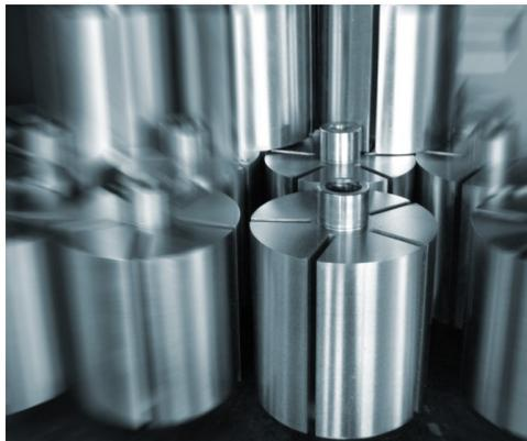
After enrichment with carbon, the steel rotor is hardened and then tempered (relaxed). During hardening the steel is heated to the austenite phase (over 723 degrees Celsius) and then quickly cooled (quenched) in order to circumvent the pearlite and ferrite phases and reach the so-called hardened martensite microstructure. The hardening procedure is followed by tempering (regulated reheating) process in order to give the steel back a certain degree of strength and ductility.
