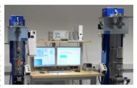
automobile industry. Therefore modern assembly tools are equipped with torque transducers which are responsible for control, documentation and recording of torque values during assembly.
