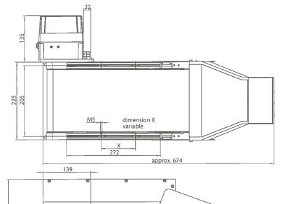
M1:10 View shows standard execution: motor position on right side
